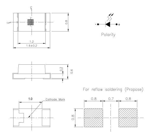
**Note:** Tolerances Unless Dimension is ±0.1mm ,Unit = mm
